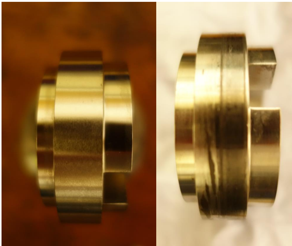
Figure 4 Repeat 1 wheel disc before (L) after (R)
