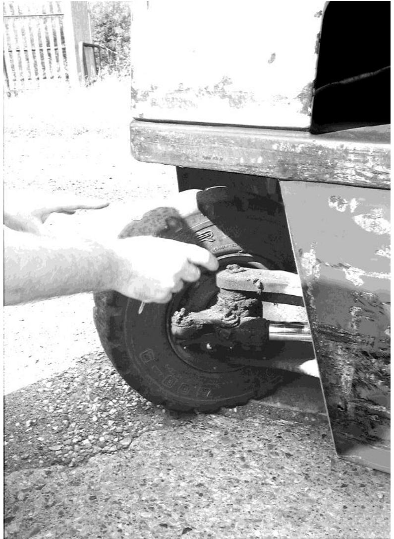
Kingpin greased with Lofrix Grease
